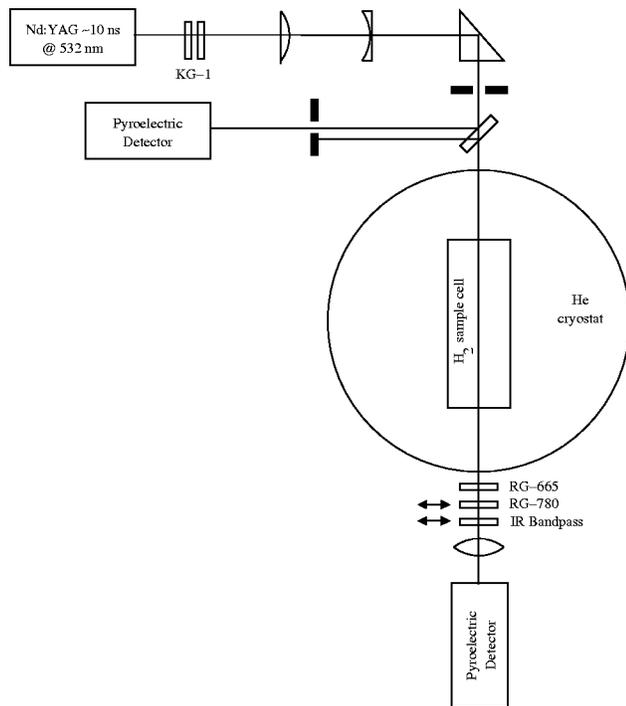
FIG. 1. Experimental configuration for Raman shifting measurements.
