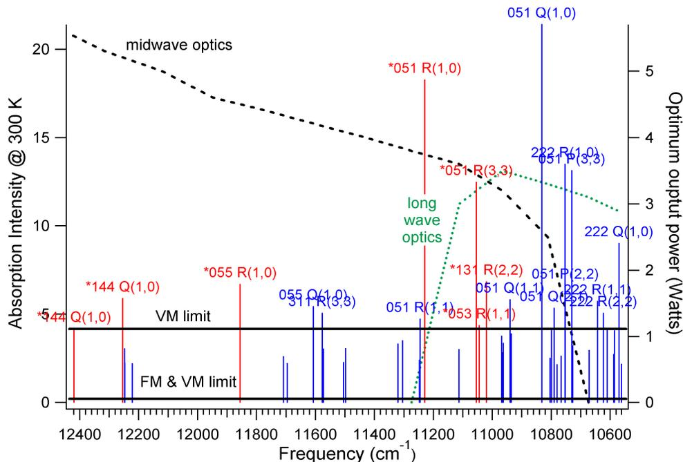
Figure 3. The tuning curves for two of the optics sets of the Ti:sapphire laser and the predicted spectrum of  $\text{H}_3^+$  overtone and combination bands above the barrier to linearity. Also shown are the experimentally determined sensitivity limit for velocity-modulated detection and the theoretical sensitivity limit for frequency- and velocity-modulated detection (described below).
