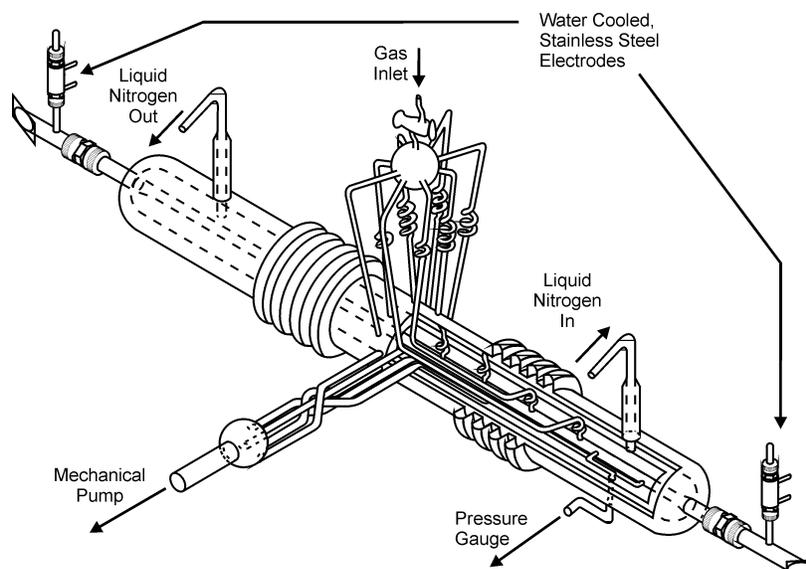
Figure 4. The liquid-nitrogen cooled discharge cell.
