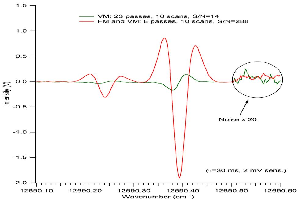
Figure 8. This figure compares the velocity-modulated signal of  $\text{N}_2^+$  and the double-modulated signal. The smallest line is the  $P_{21}(16)$  transition of the  $(2,0)$  vibrational band of the Meinel system  $\text{A}^2\Pi_u-\text{X}^2\Sigma_g^+$ , while the larger signal is the  $Q_{22}(16)$  transition. The signal-to-noise ratios were calculated from the  $P_{21}(16)$  transition – which is comparable in intensity to the  $5\nu_2$   $R(1,0)$  line of  $\text{H}_3^+$ .
