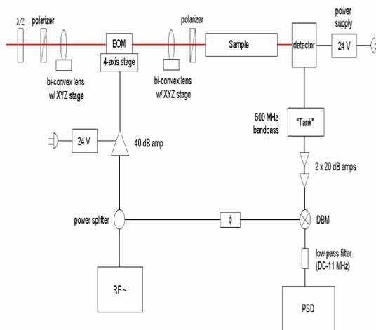
Figure 5. Schematic of the heterodyne detection electronics.
