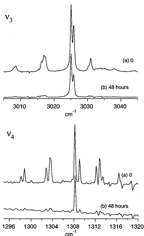
FIG. 4. Temporal dependence of the FTIR spectra of methane trapped in solid parahydrogen. The upper and lower panels show the  $\nu_3$  and  $\nu_4$  fundamental bands, respectively. In each panel traces (a) and (b) show the spectrum observed immediately after the growth of the crystal and after 48 h standing at 4.8 K, respectively.
