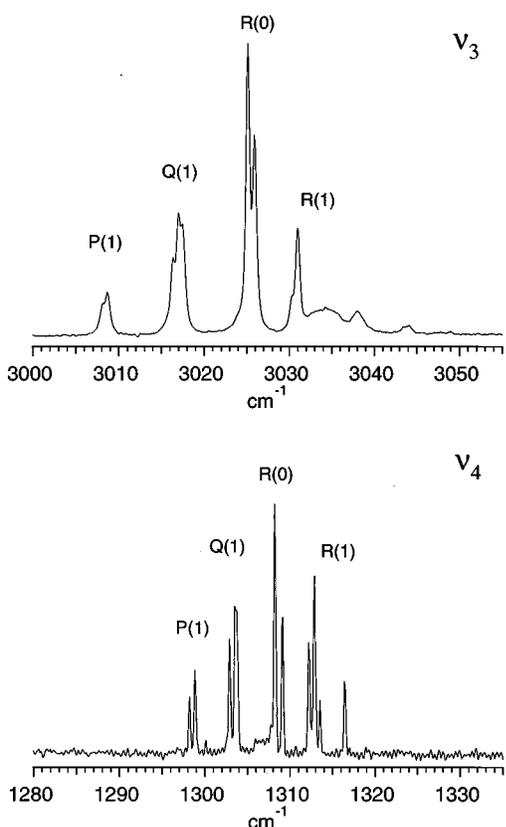
FIG. 2. FTIR spectra of methane trapped in solid parahydrogen. (a) The  $\nu_3$  fundamental band. (b) The  $\nu_4$  fundamental band. The spectral resolution is  $0.25 \text{ cm}^{-1}$ . The linewidths of the  $\nu_3$  and  $\nu_4$  transitions are about  $1 \text{ cm}^{-1}$  and  $0.25 \text{ cm}^{-1}$  (limit of the spectrometer), respectively.
