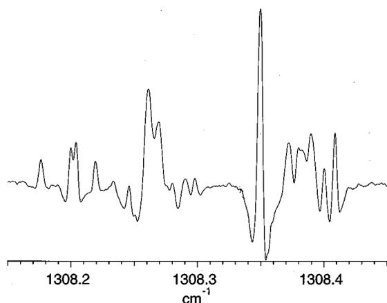
FIG. 6. High resolution spectrum of the R(0) band at 1308.25 and 1308.37  $\text{cm}^{-1}$  in Fig. 1. The spectrum was observed after a prolonged standing beyond 48 h. The tone-burst modulation technique with a rf sideband of 60 MHz was applied. The linewidth is as narrow as 0.003  $\text{cm}^{-1}$  (100 MHz).
