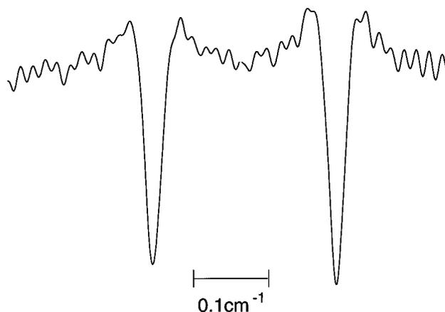
FIG. 3. High resolution laser spectrum of part of the  $\nu_4$  transition of methane at 1303.7  $\text{cm}^{-1}$  in Fig. 2(b). The spectrum was observed by the tone-burst modulation technique with a rf sideband of 100 MHz. The figure shows that the barely split doublet (actually appearing as a blunted singlet) at around 1303.7  $\text{cm}^{-1}$  in Fig. 2(b) consists, in fact, of two lines with linewidths of 0.027  $\text{cm}^{-1}$  (FWHM).
