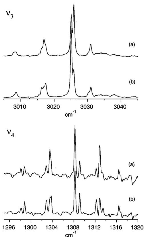
FIG. 5. The polarization dependence of the FTIR spectrum of methane trapped in solid parahydrogen. The upper and lower panels show the  $\nu_3$  and  $\nu_4$  bands, respectively. In each panel traces (a) and (b) show the spectrum when the polarization of radiation is in parallel with and perpendicular to the  $c$  axis, respectively.
