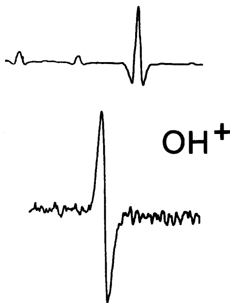
FIG. 2. The rotational transitions N = 13 \leftarrow 12 , F_3 \leftarrow F_3 of \text{OH}^+ . The time constant of lock-in detection is 1 s. The upper trace is \text{CS}_2 reference spectrum.
