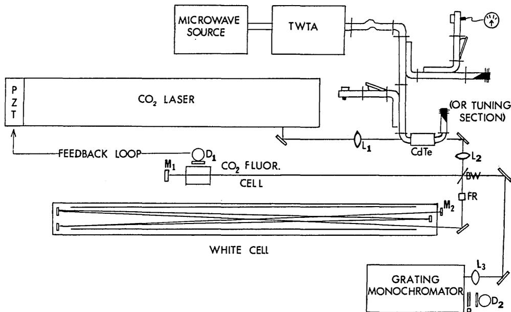
Fig. 1. Experimental setup.  $L_1$ – $L_3$ , ZnSe lenses;  $M_1$ , reflection mirror mounted on a speaker;  $M_2$ , plane reflection mirror;  $D_1$ , InSb detector;  $D_2$ , HgCdTe detector; BW, Brewster-angle window; FR, Fresnel rhomb; P, grid polarizer; TWTA, traveling-wave tube amplifier; PZT, piezoelectric translator.
