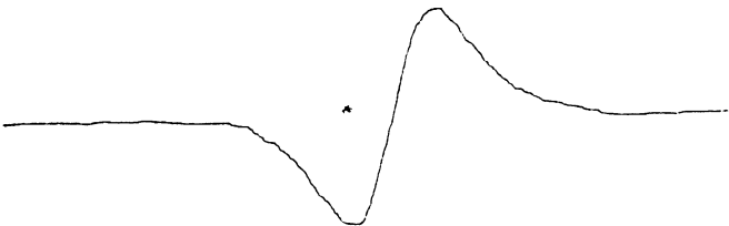
FIG. 2. The double resonance signal. The pressure was 20 m torr. The cavity resonance was tuned to 423.02 MHz. The sweep covers about 3 MHz. The PSD time constant is 3 msec. This trace is the average of 128 sweeps in a total time of 34 sec.
